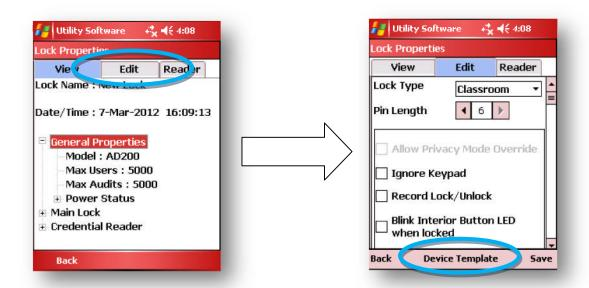
3. Tap on Device Template menu, (shown above) and select the "Save to Device" option, then select the Device Template you want to load into the device and tap "OK." This Device Template file of "Lock Properties" will be loaded and saved on this lock/device. Only Device Templates that match this device hardware type will be presented to select. (For an AD200 PROX you will not see AD200 MAG templates)
