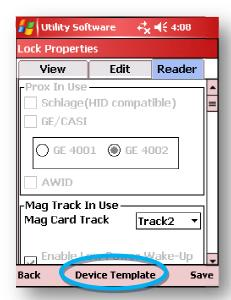
NOTE: The *Device Template* can be selected from either the "Edit" or "Reader" tabs. Saving or Restoring a *Device Template* from either screen will update ALL device settings, not just the "Edit" or "Reader" screen options.
