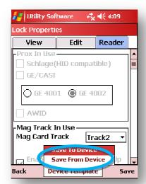
B. Tap on the "Save From Device" menu option to bring up the screen below. This will copy the lock properties from this device (lock or module) into the SUS file.
